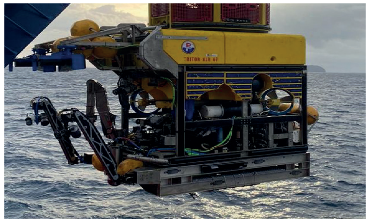
ROV XLR-07 fitted with INS, MBES, SSS, SBP, Cable Tracker & Video
